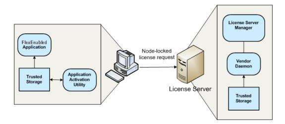
Figure 2-2: FlexEnabled components for trusted storage on a network machine
