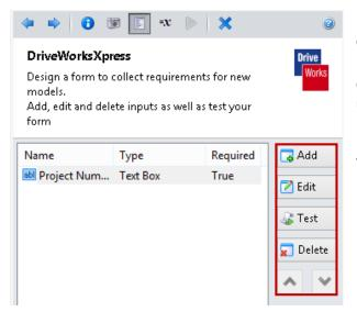
Notice that the form control appears in the form designer within the DriveWorksXpress Task Pane. As you create your form, you can edit and delete controls, as well as change the order by using the Up and Down arrows.
