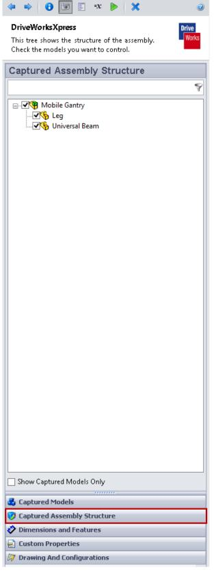
At the bottom of the Task Pane, select the 'Captured Assembly Structure' tab. This will display check boxes next to each model in the assembly. Select the parts/assemblies that you want DriveWorksXpress to control by checking the box next to each item.
