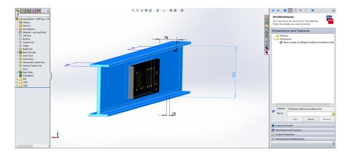
In the SOLIDWORKS Feature Manager double click the feature Base Extrude. The section height dimension will appear on the model.
