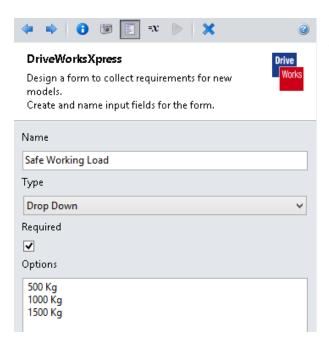
NOTE: These values will drive a configuration in the Universal Beam. Ensure that the entries are identical to those shown (spaces between 0 and K, upper case K and no spaces at the start or end of each text string.
