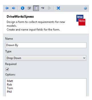
NOTE: Separate items in the Options field of the Drop Down by using pipe bars (Matt|Rob) or by pressing Ctrl+Enter after each entry to add a new row.
