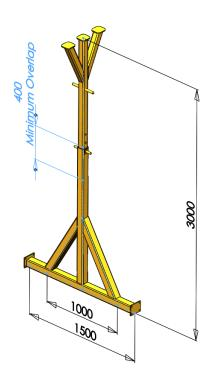
The overall width of the mobile gantry may also affect whether or not we need all the supporting members. DriveWorksXpress can control the suppression state of SOLIDWORKS sketches, planes, features etc.
