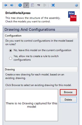
Open the Mobile Gantry assembly and browse for the drawing 'Mobile Gantry.SLDDRW'.
